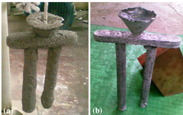
Fig. 1 Cast cp-Ti bars by investment casting. (a) Ceramic mold and (b) cast bars
